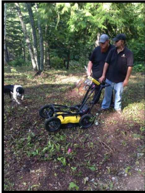
Figure 5.6. Maverick Inspections Ltd. using the GPR in the Morrissey Cemetery
